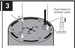
Measure 3 x suspension wires and mains cable to required length and carefully trim.
