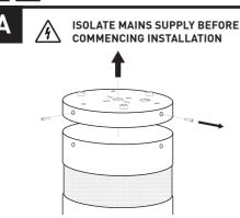
Remove the three screws and then the lid.
