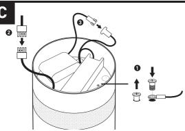
• Remove screw and attach wire tether using same screw.
