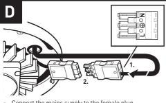
Connect the mains supply to the female plug (supplied) (1), then connect the female plug to the male plug on the luminaire (2).
