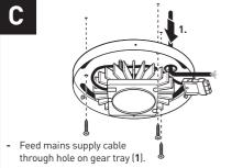
Replace gear tray on mounting surface and fix to ceiling securely using suitable fixings (not supplied).
