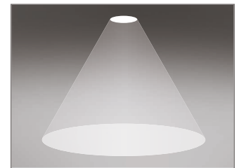
/WB 60° wide beam reflector
