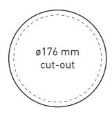
Cut a 176 mm circular hole at the desired location using a holesaw.
