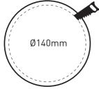
Cut a Ø140mm circular hole at the desired location using a holesaw.
