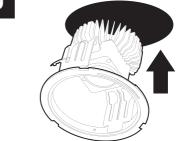
Insert luminaire into the ceiling void.
