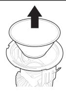
Remove reflector from luminaire taking care not to damage the reflector's surface.
