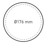
Cut a 176 mm circular hole at the desired location using a holesaw.
