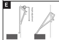
Lock the luminaire in place by means of the four adjustable fixing springs as illustrated above.
