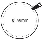
Cut a 140 mm circular hole at the desired location using a holesaw.
