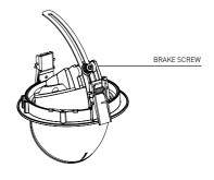
Adjust the luminaire head to the required position. The head resistance can be adjusted using the brake screw if necessary.
