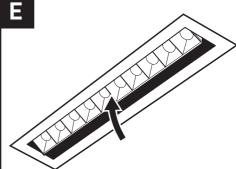
Tilt the luminaire head to the required position by pushing in the centre. (Not IP65 Version)
