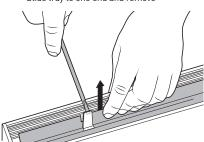
Disconnect the driver connectors and the earth spade to release the downlight LED trav.
