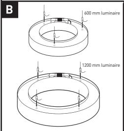
Screw suspension clutches on to studs on the back of luminaire. Three suspension clutches for 600 mm luminaire or four for 1200 mm luminaire.
