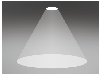
/WB Wide beam reflector 36.2°
