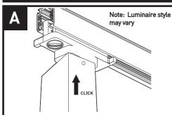
Push spotlight up into the track, listening for the click. The spotlight can only be fitted one way, ensure to check polarity first. - DO NOT FORCE
