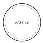
Using a holesaw, cut out a ø73 mm hole on a flat, smooth surface at the required location. В
