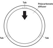
Carefully release the securing tabs to remove the diffuser.
