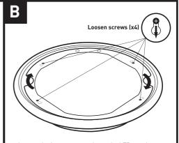
Loosen the four screws and turn the LED panel to release. Lift and remove the gear tray assembly.
